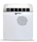
The call unit is activated when we press the call button, the receiver will emit a sound and a flashing light, indicating that a visitor needs assistance.
