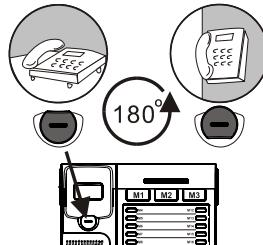
Install two screws at a distance of 83 mm from each other on a vertical line. Leave the screws protruding from the wall by 5mm.
