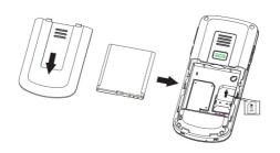
Observe the battery contacts (the gold coloured contacts must face towards the bottom right).and insert the battery.
