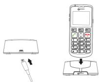
**Note:** Only use batteries and chargers supplied with the telephone. The guarantee will be invalid if an unapproved cable is used. Keep the battery contacts clean and free of dirt. Try and avoid removing the battery as this could short circuit the battery.
