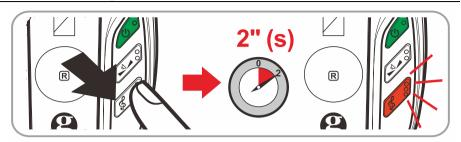
The tone can be controlled by pressing the tone button on the headphones. Press and hold this for 2 seconds, the button will light up red. At this point, pushing headset '+' button will increase the high tones. Pushing the '–' button will increase the low tones. At minimum, maximum or middle point a beep will be heard. If the buttons are not pressed, tone setting mode will switch off automatically after 5 seconds.
