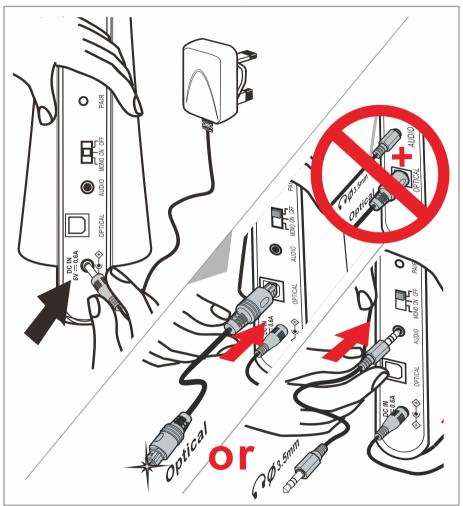
2. Insert one end of the 3.5 mm jack cable into **AUDIO** socket on the back of the charging base, or insert the one end of optical cable into the **OPTICAL** socket on the back of the charging base.
